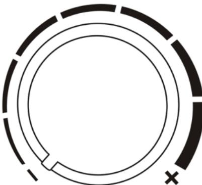
Then select the desired temperature using the "Temperature controller". "Minus (-)" is the lowest temperature setting and "Plus (+)" is the highest. To switch off the appliance completely, disconnect the mains plug from the socket.
